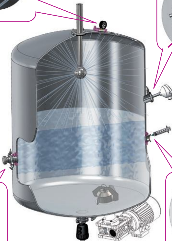
Traditional Triclamper connectors are hard to clean by spray ball
