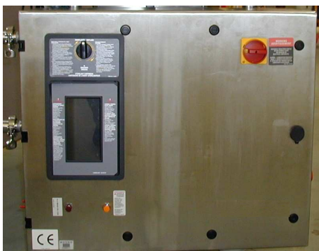
In this picture, a vapor generator for hydrogen peroxide H 2 O 2 (VHP®)
