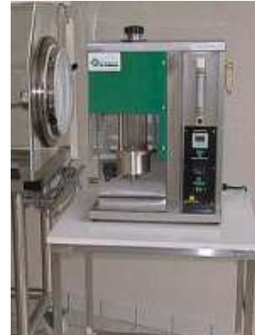
In this picture, a vapor generator for peracetic acid PA (MAN)
