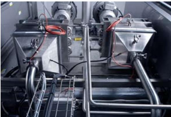
Exclusive twin channel drying system. Each channel comprises a high capacity blower powered by a brushless fan, a heating system (electrically heated ceramic element as standard, steam heating as option) and a HEPA filter (in that sequence). One channel is used to dry the chamber and load exterior whilst the other assures rapid drying of the hydraulic circuit, rack and load interior.
