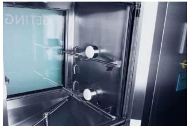
Doors slide or are hinged to provide convenient and ergonomic loading while optimising space usage (overall footprint) and ergonomics. All doors comprise of two sheets of toughened tempered glass, with an air gap providing heat and noise insulation. The glass door allows visual monitoring of the cleaning action – e.g. spray arm rotation, facilitating qualification. Optional chamber illumination.
