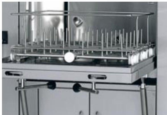
Doors fold down to provide convenient and ergonomic loading. The operation is assisted by gas-dampened supports that reduce the effort required by the user. On larger models, legs fold out to support the open door, while on smaller models, the supports are anchored to the machine frame, as shown here.
