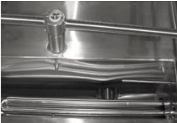
A sanitary steam heating coil in the sump rapidly heats circulating water and accurately controls the temperature. If steam is not available, electrical heaters may be provided in the same location.
