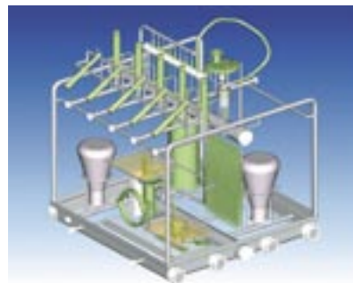
3D CAD modeling is used to design tailor-made racks for different applications, usually in cooperation with the user or equipment supplier.
