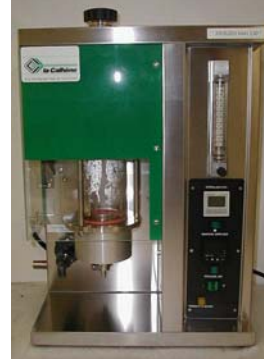
Vapor generator for peracetic acid PA (MAN)
